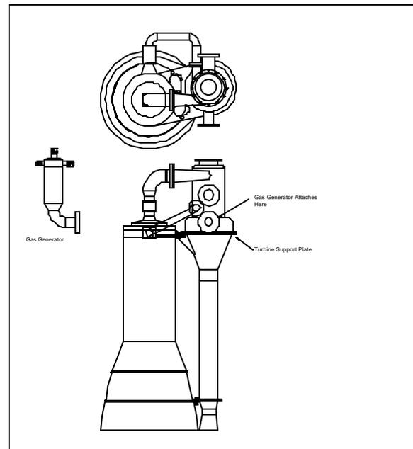
Propellant for the first stage gas generator is held in three small spherical fuel tanks and one oxidizer tank. In the second stage, two unequal sized tanks hold fuel and oxidizer. All gas generator tanks are filament-wrapped graphite-epoxy spheres pressurized to 1400 PSIA.
