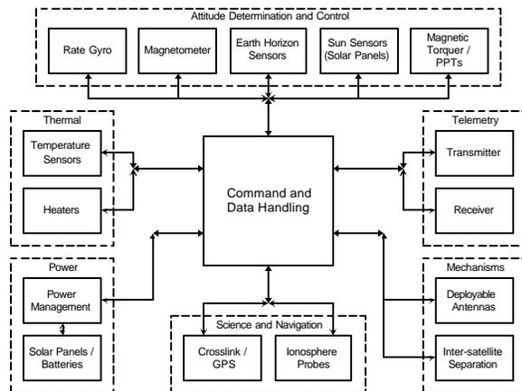
**Figure 2. System-level interface diagram for C&DH subsystem.**
