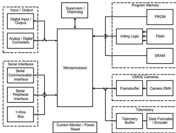
**Figure 3. Top-level interface diagram for C&DH subsystem.**
