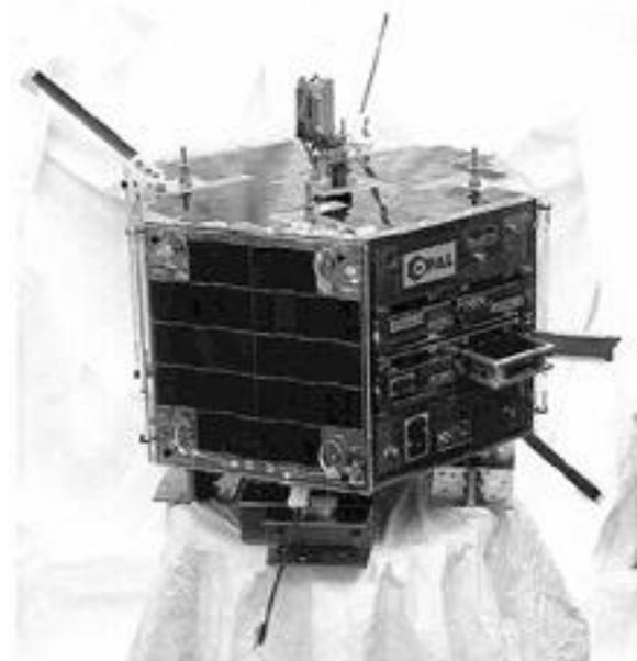
Figure 4 – OPAL complete with picosatellite in launch tube.
