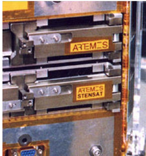
Figure 6 – Head on view of two picosatellite tubes.
