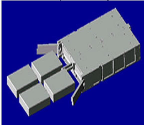
Figure 5 – Rendering of two launch tubes.
