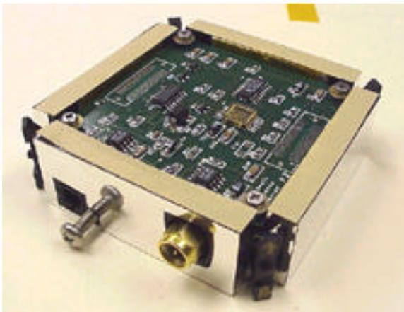
Figure 10 – Inner electronics of an Aerospace picosatellite.
