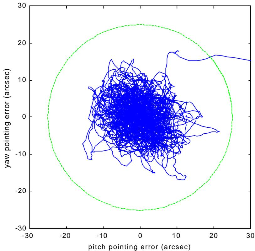
Figure 4: Telescope boresight pointing error for MOST
