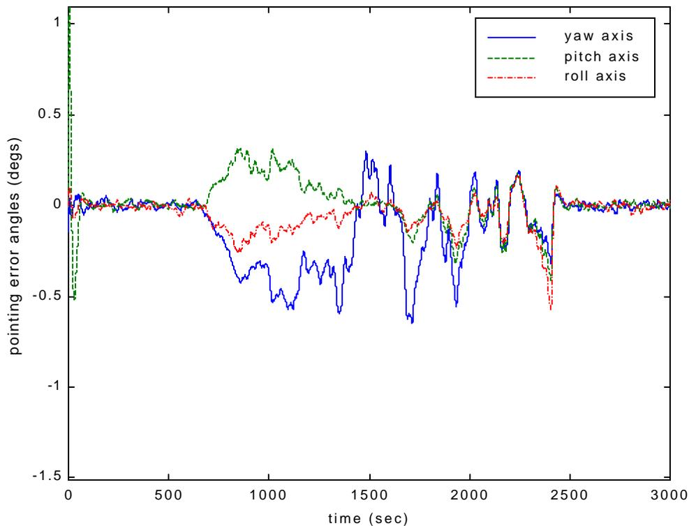
Figure 2: Pointing accuracy for CHIPSat through eclipse
