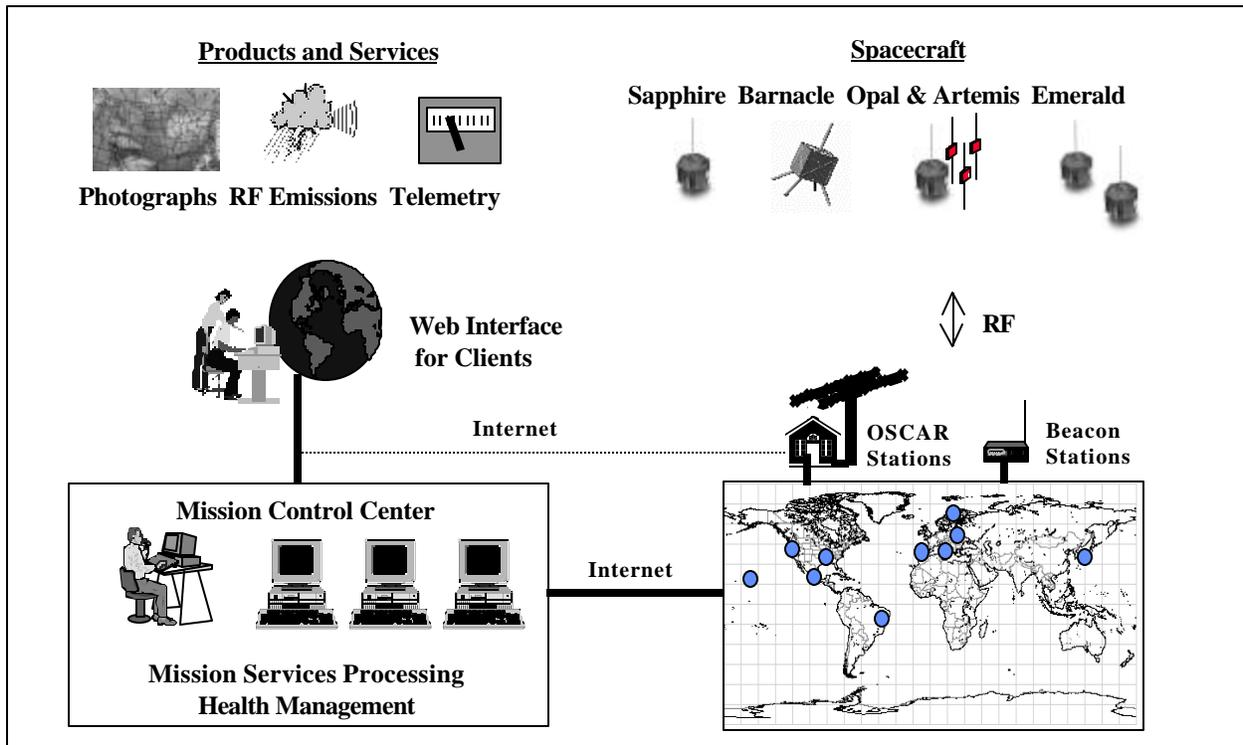
Figure 4. The Mission Control Architecture
