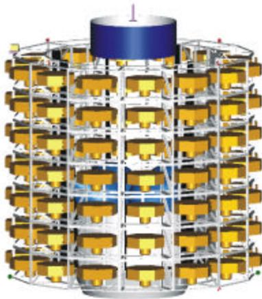
**Figure 2. Nanosatellite Deployer Ship Concept**
