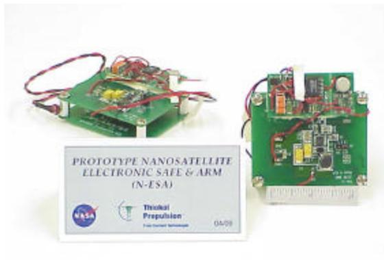
**Figure 11. Breadboard N-ESA**
