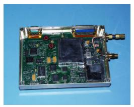
Figure 3. S-Band Down-link Module
