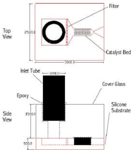
**Figure 9. MEMS Thruster Integration**
