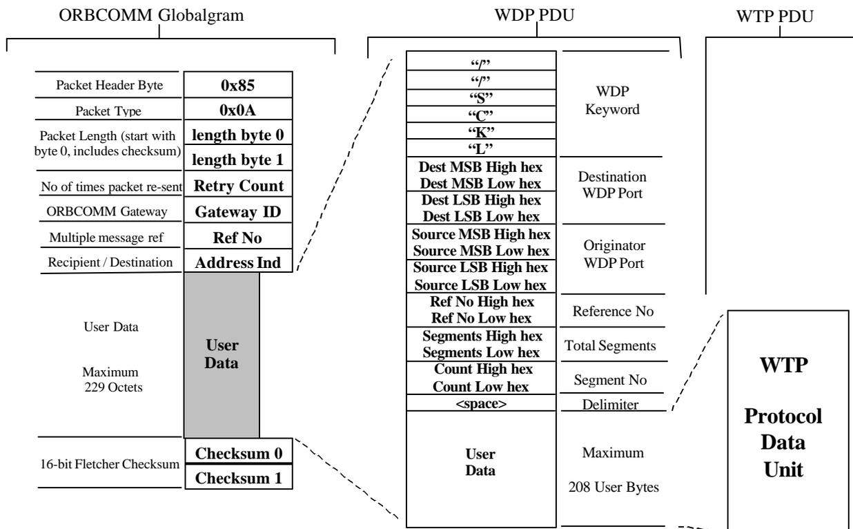
**Figure 6: SC Protocol Data Units (PDU).**
