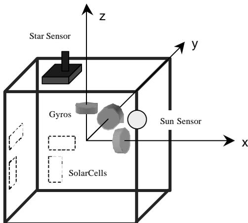
Figure 23: Baseline Sensors Layout of the LunarSat ADCS
