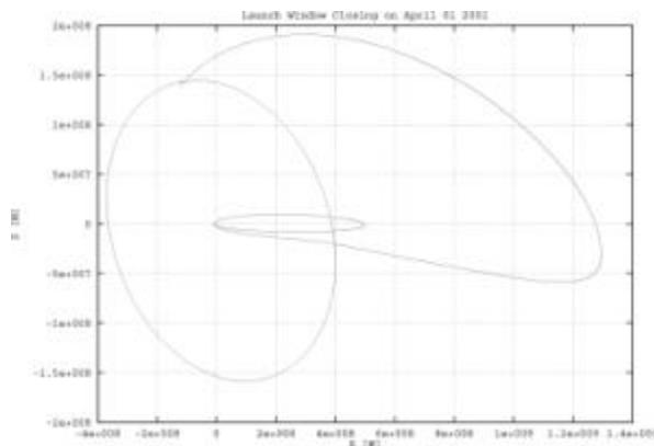
Figure 13: X-Z View of a WSB-Swing-By Transfer
