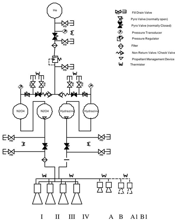
Figure 16: Design Baseline of the Propulsion System
