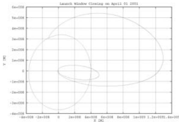
Figure 12: X-Y View of a WSB-Swing-By Transfer
