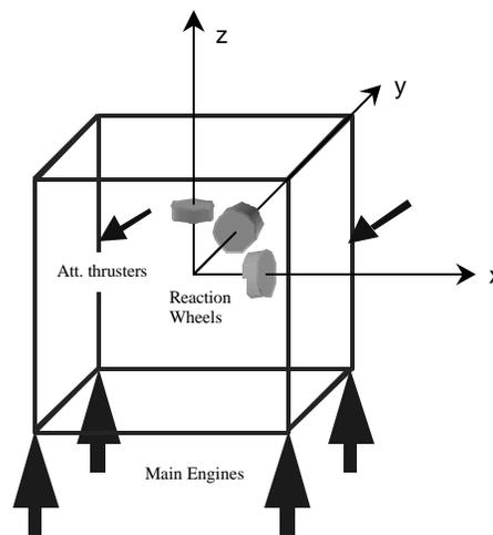
Figure22 : Baseline Actuators Layout of the LunarSat ADCS
