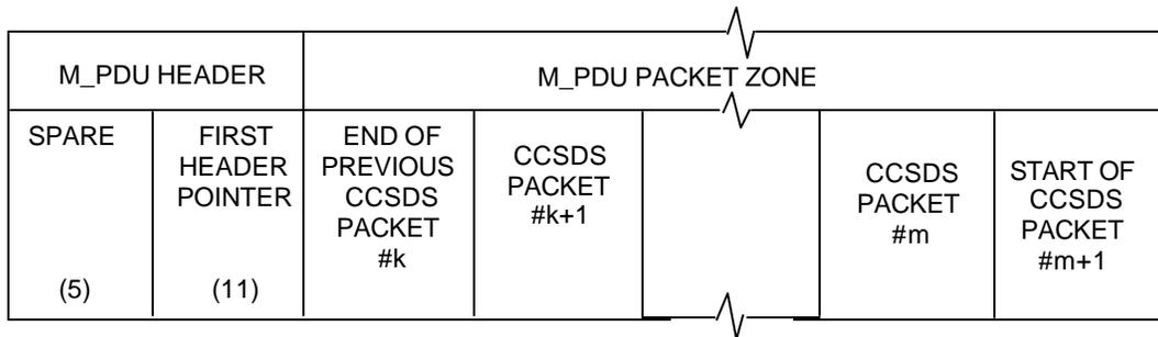
**Figure 6 – Multiplexing Protocol Data Unit Format**
