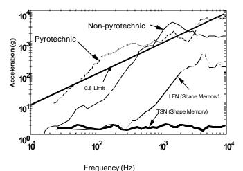
Figure 3. Comparison of Release Device Shock Output <sup>2</sup>
