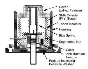
Figure 2. Two Stage Nut Cutaway (Lockheed Martin Astronautics)
