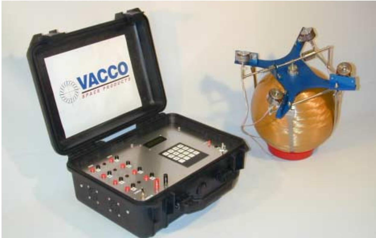
**Figure 10:** Cold Gas Propulsion System Test Specimen and Control Box
