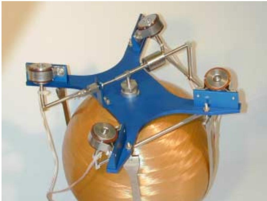
**Figure 5: Cold Gas Propulsion Demonstration System**
