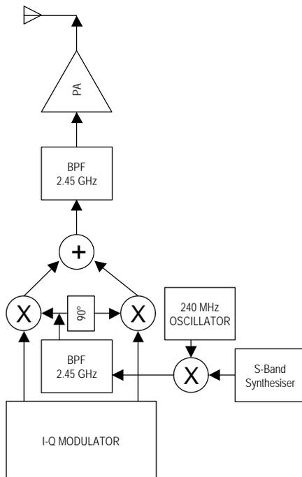
Figure 10 Modified Direct Up Conversion IQ Modulator
