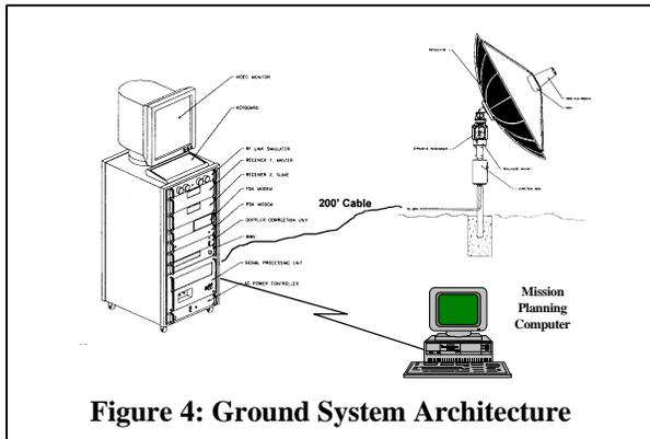
**Figure 4: Ground System Architecture**
