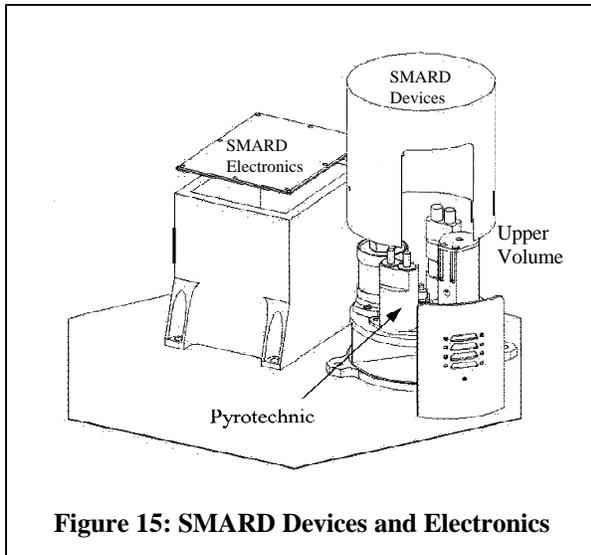
**Figure 15: SMARD Devices and Electronics**
