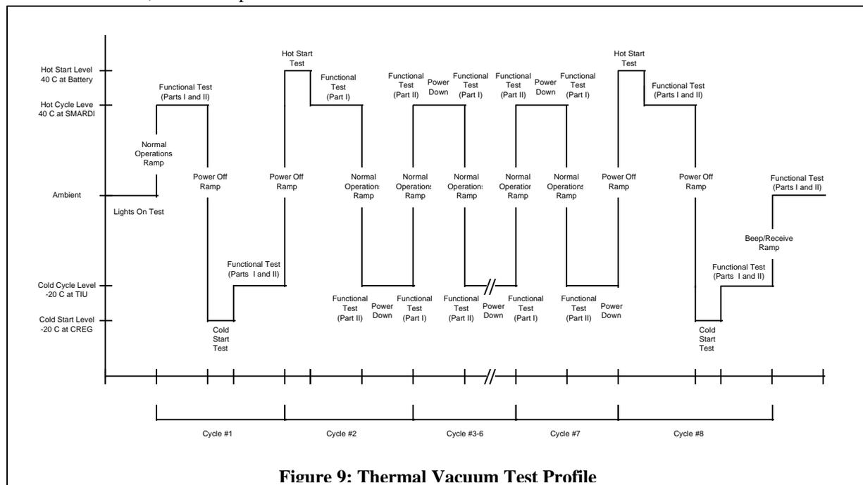
**Figure 9: Thermal Vacuum Test Profile**
