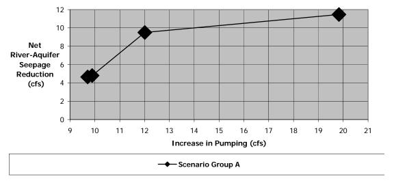
**Fig 4** Trade-off curve of groundwater pumping increase versus net river-aquifer seepage decrease. (To convert cfs to m<sup>3</sup>s<sup>-1</sup> multiply by 0.0283.)
