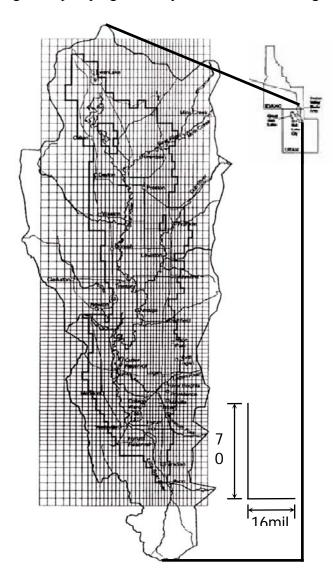
**Fig 3** Cache Valley location in Utah and Idaho, and groundwater model grid (from Kariya, et al., 1994).
