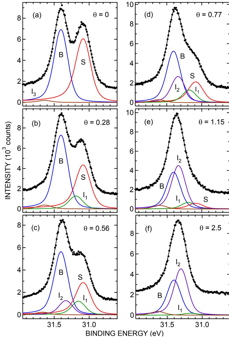
FIG. 2 Least-squares analysis of W  $4f_{7/2}$  core level spectra from the Ni/W(110) bimetallic interface. Peaks due to bulk W (B), clean-surface W (S), and W atoms covered by  $1 \times 1$  ps Ni ( $I_1$ ) and  $8 \times 1$  and  $7 \times 1$  cp Ni ( $I_2$ ) are shown. A third, much smaller interface peak [ $I_3$  in (a)] is also shown. Indicated coverages of Ni are in units of a ps ML.
