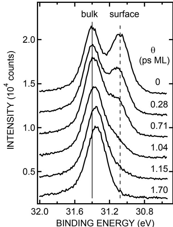
FIG. 1 W $4f_{7/2}$  core level spectra from the Ni/W(110) bimetallic interface, illustrating the effect of increasing Ni coverage. The solid and dashed lines mark the positions of the bulk and clean-surface core-level features, respectively.
