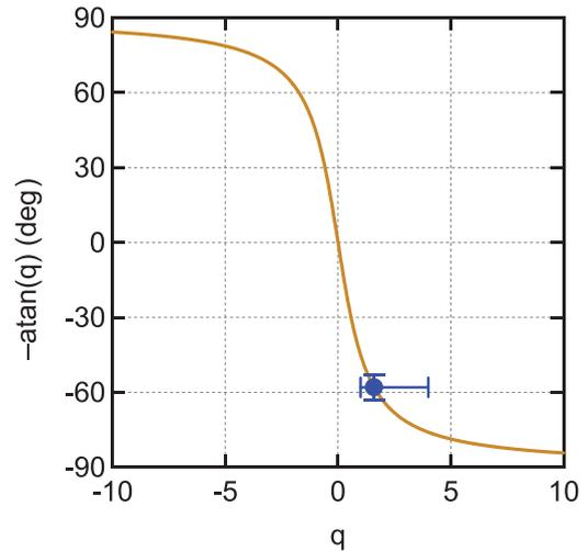
FIG. 2. (Color online) Phase  $\phi = -\text{atan}(q)$  vs  $q$  for the classical Fano oscillator. The solid circle (with vertical error bars included) is the phase that has been measured for a degenerate  $p$ -type Si sample ( $p$  between  $3 \times 10^{19}$  and  $1.5 \times 10^{20} \text{ cm}^{-3}$ ),<sup>18</sup> the horizontal line spans the range of estimated  $q$  values for the sample as deduced from Fig. 3 (see text for details).
