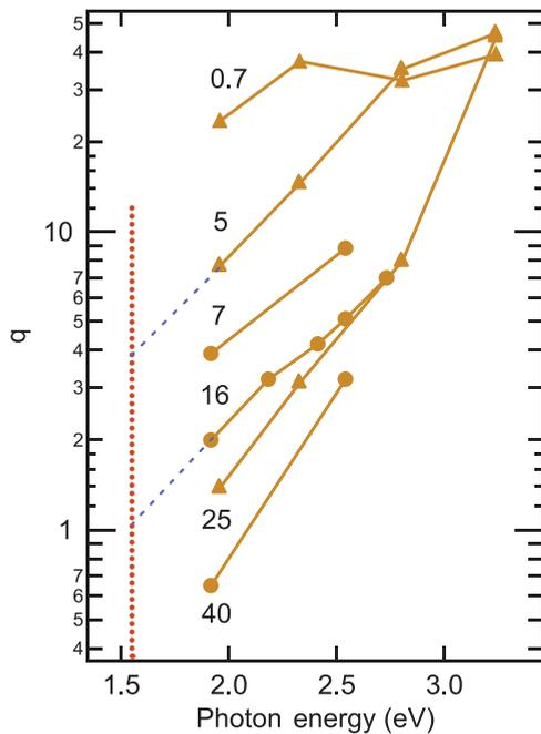
FIG. 3. (Color online) Experimental Fano asymmetry parameter  $q$  deduced from Raman-scattering data vs photon energy  $\hbar\omega$  for degenerate  $p$ -type Si. Indicated doping density for each curve is in units of  $10^{19} \text{ cm}^{-3}$ . Triangles are from Ref. 8, and circles are from Ref. 7. Dotted lines are extrapolations of the  $5 \times 10^{19}$  and  $1.6 \times 10^{20} \text{ cm}^{-3}$  data to  $\hbar\omega = 1.55 \text{ eV}$ .
