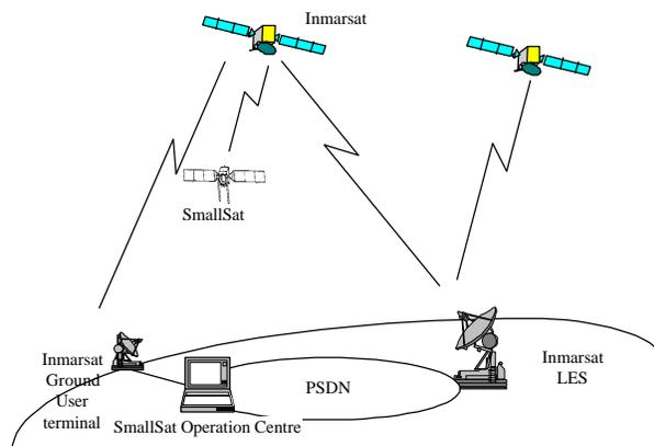
Fig. 2 The proposed system architecture for SmallSat Data Relay and Control
