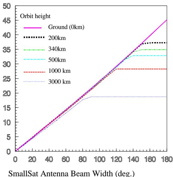
Fig. 1 the impacts of SmallSat antenna beam on orbit coverage rate (for one Geo. Satellite)
