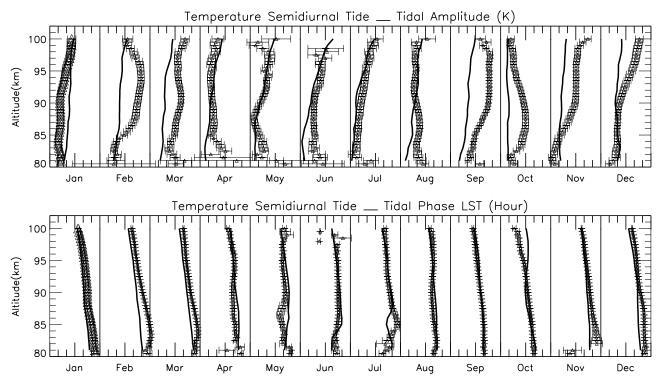
**Figure 1.** Temperature semidiurnal tidal (top) amplitude and (bottom) phase profiles for each month of the year measured by Na lidar (triangles with error bars) and HAMMONIA (solid lines). Each amplitude scale (horizont s) is 0-15 K, and each phase scale (horizontal axis) is 0-18 h.
