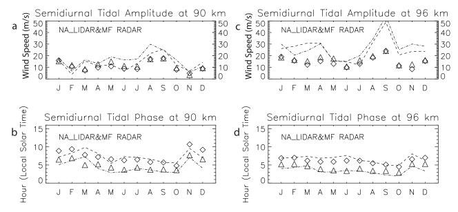
**Figure 4.** Semidiurnal tidal amplitude and phase comparison between the Colorado State University Na lidar-observed zonal wind (dashed line) and meridional wind (dash-dotted line), and MF radar (Urbana, Illinois) observed zonal wind (diamonds) and meridional wind (triangles): (a and b) for 90 km and (c and d) for 96 km.
