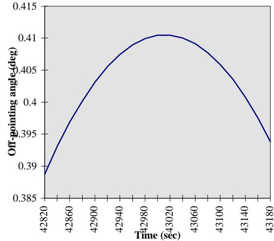
Figure 5 . UoSAT Microsatellite mispointing plot 360second period
