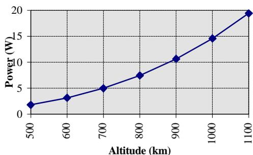
Figure 9. Satellite altitude vs. required transmitted power
