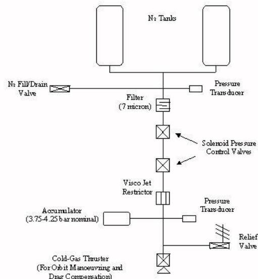
Figure 7. MicroBus cold gas station keeping system
