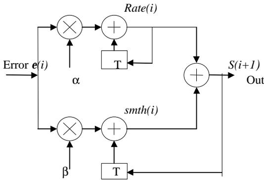
Figure 4. **a-b** filter diagram
