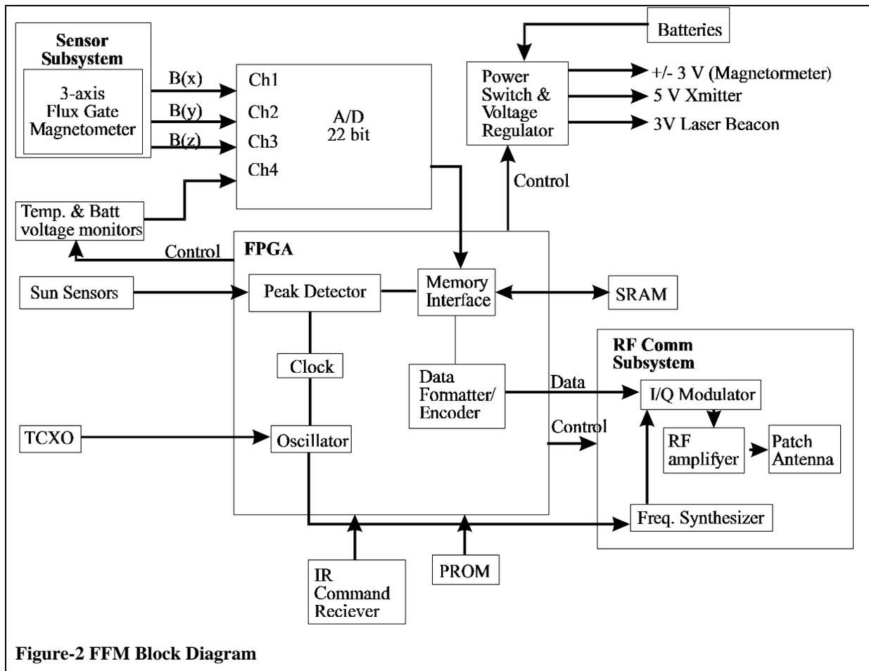
Figure-2 FFM Block Diagram
