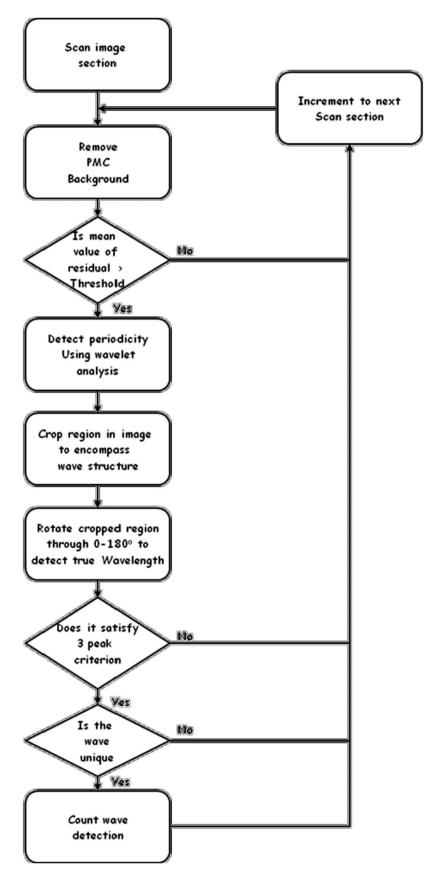
Figure 3. Graphical depiction of wave detection algorithm.
