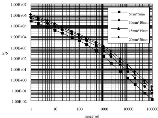
Fig.7 Signal-to-Noise Ratio of MS-LRF for CCR Target
