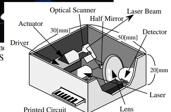
Fig.2 Concept of Micro-Scanning Laser Range Finder (MS-LRF).
