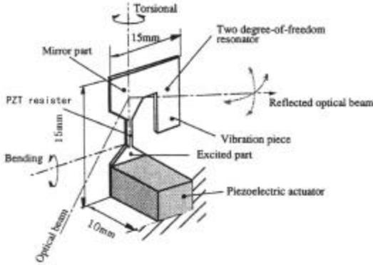
Fig.4 Structure of Micro Two-Dimensional Scanner.
