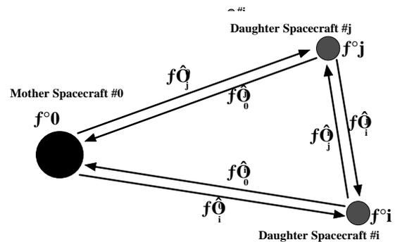
Fig.10 Attitude Determination by MS-LRFs.
