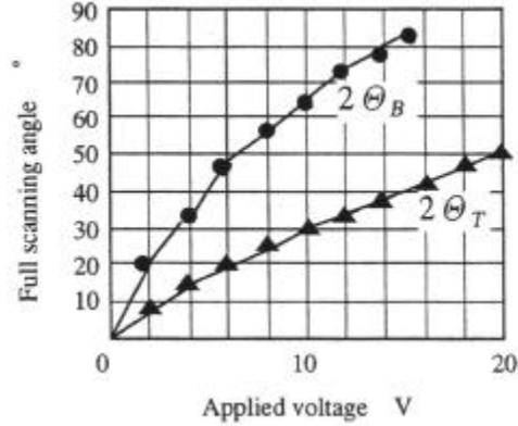
Fig.5 Full Angle of Beam Scanning by Micro-Scanner.
