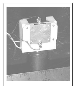
Figure 7. Colloid Microthruster Prototype
