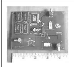
Figure 6. The Modified Mitel GPS Receiver
