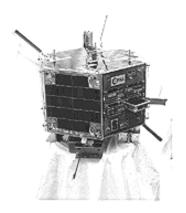
Figure 2. The Stanford Opal Microsatellite
