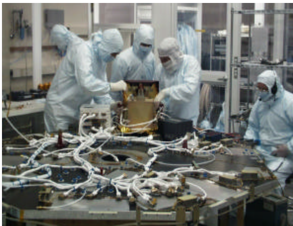
Figure 9 Photograph of payload integration and test activities at Southwest Research institute (SwRI). The instrument being integrated is the High Energy Neutral Atom Imager (HENA), developed for IMAGE by the Applied Physics Laboratory (APL).
