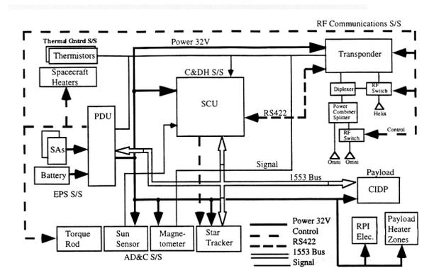
Figure 7 IMAGE Observatory simplified electrical block diagram.
