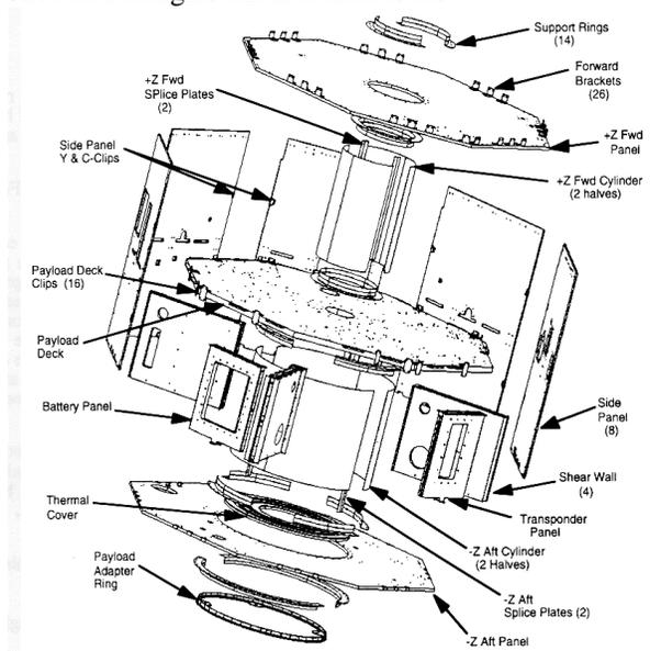
**Figure 3 Exploded view of the IMAGE spacecraft structure.**
