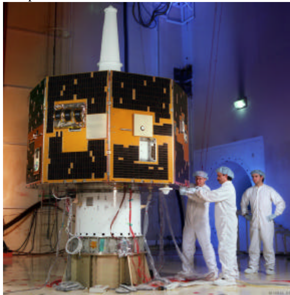
Figure 1 Photograph of the assembled IMAGE Observatory in preparation for vibration tests. (Photo courtesy of Lockheed Martin Missiles & Space Company).
