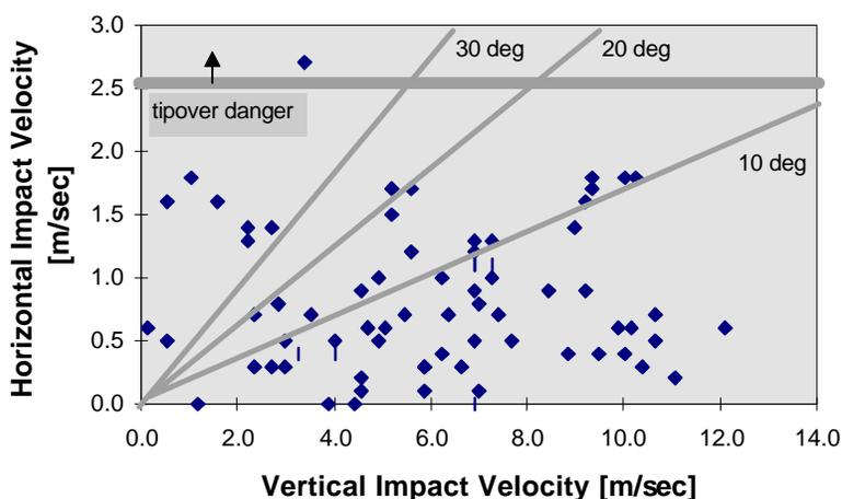
**Fig. 5. Preliminary results of 6-DOF Monte-Carlo simulations shows the surface impact vertical and horizontal velocities are within the expected range.**
