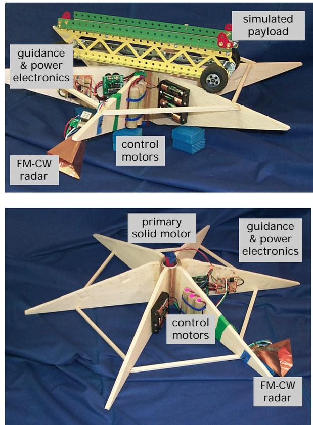
**Fig. 6ab.** Functional Microlander breadboard is intended for benchtop testing. It will be soon upgraded with full complement of sensors and motors and field tested. The upper photo shows the simulated payload. The microlander is inverted in the lower photo to show primary motor (scaled for terrestrial terminal velocity).
