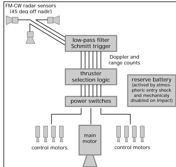
**Fig. 2. Microlander Electronics Block Diagram shows the fundamental simplicity of this Mars microlander design**
