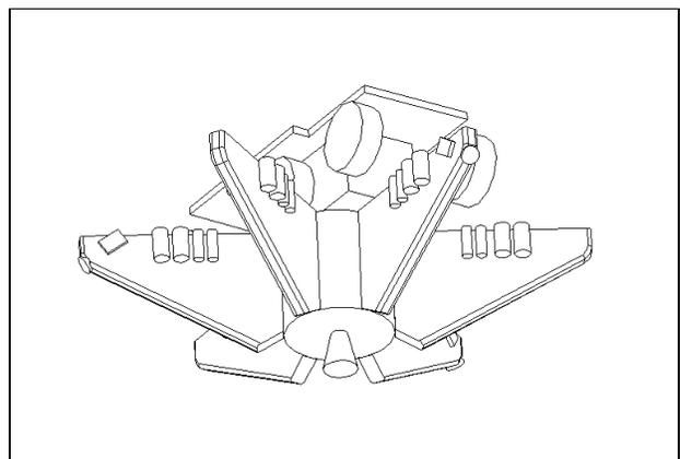
**Fig. 4ab. Microlander structure supports main and control motors, guidance sensors, microlander electronics and payload.**
