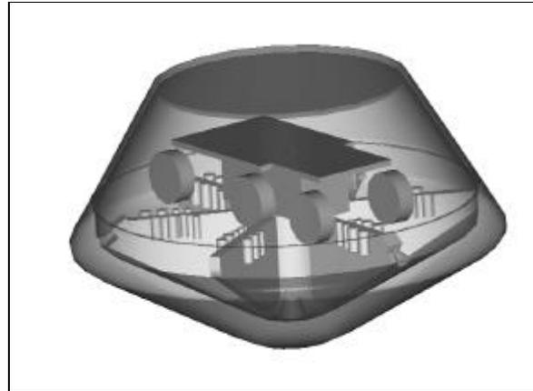
**Fig. 3. Microlander proper is located in the bottom half of the Stardust-shaped aeroshell (front shell). Payload (a small rover in this picture) is located in upper half of aeroshell (aft shell). The combined CG location is approximately at mid-point between two shells.**
