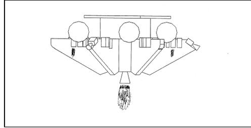
8) *The microlander impacts the surface.* Some of the impact shock is absorbed by the microlander structure. The microlander structural ribs are made from the crushable material and the primary motor nozzle can collapse inside the motor chamber. This microlander impact shock absorption limits the payload impact shock to under 500 Gs. The surface impact also inhibits (by interrupting the battery power) the microlander electronics so additional control motor firings are disabled.
