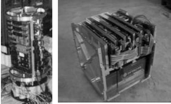
Figure 1. The Barnacle Microsatellite a) sounding rocket configuration (left) and b) orbital configuration (right).
