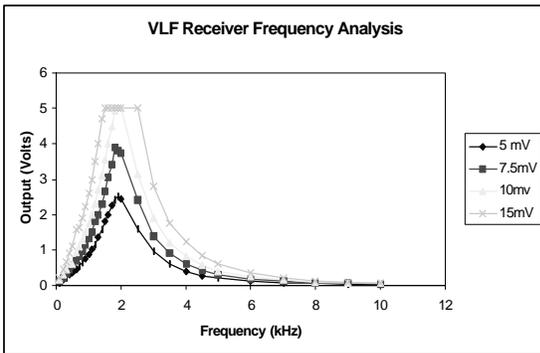
Figure 7. VLF Receiver Frequency Analysis
