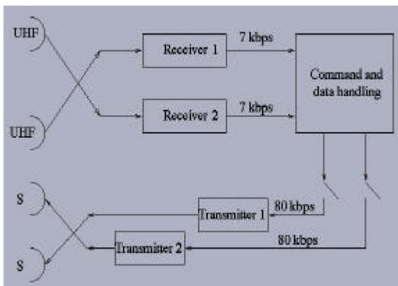
**Figure 7.2 – Communications Block Diagram**
