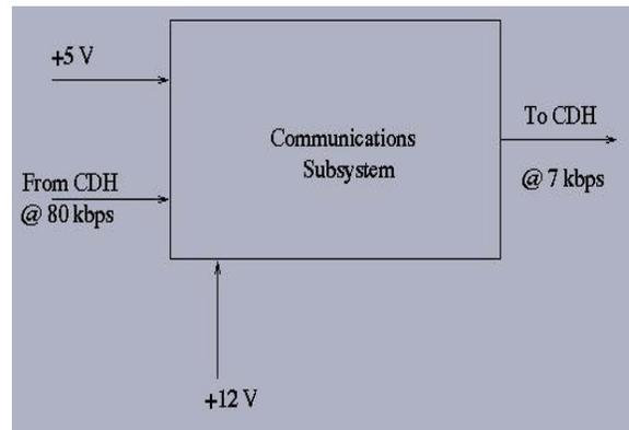
**Figure 7.1 – Communication System Architecture**
