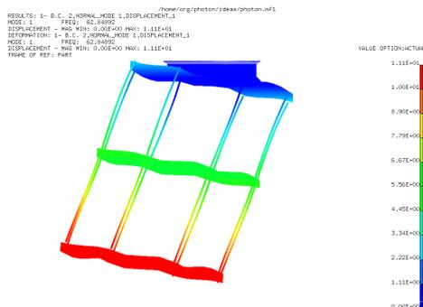
Figure 3.6 – First Mode Shape (exaggerated deflection)
