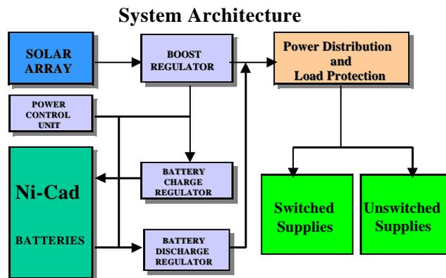
**Figure 8.1** – Power Distribution Architecture
