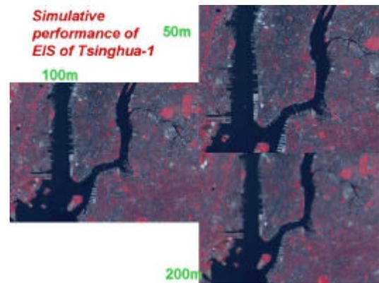
Fig. 5 The simulating performance of Tsinghua-1 MEIS with 50m ground resolution.
