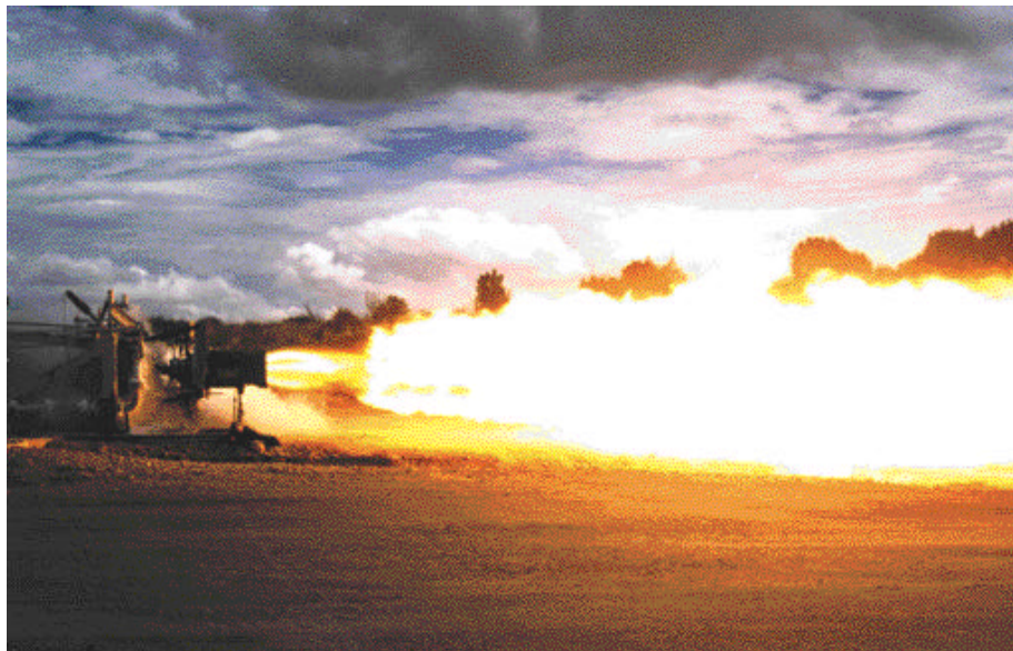
Figure 4. Testing of 40,000-lb. Thrust Engine at the Rocket Propulsion Test Facility. These tests were used to characterize a 40,000-lb. thrust injector modified by TRW for the Scorpius™ program.
