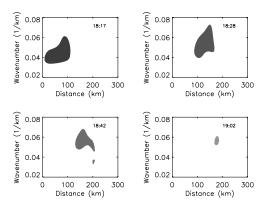
**Figure 5.** Contours of the spatial S-Transform amplitudes (wave number vs southward distance) at four different times. As the wave packet evolves, the horizontal wave number increases. Also, the wave packet can be seen to move into the field of view (distance = 0 km) but the amplitude dies out and it does not leave the field of view (distance = 300 km).
