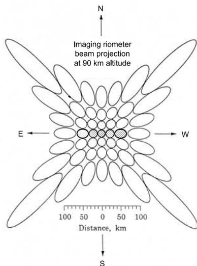
**Figure 1.** The projection of the imaging riometer beams onto a horizontal plane at 90 km altitude, as defined by their beam 3dB power contour [adapted from *Detrick and Rosenberg, 1990*]. The central east-west line of five beams discussed in the text are shaded.
