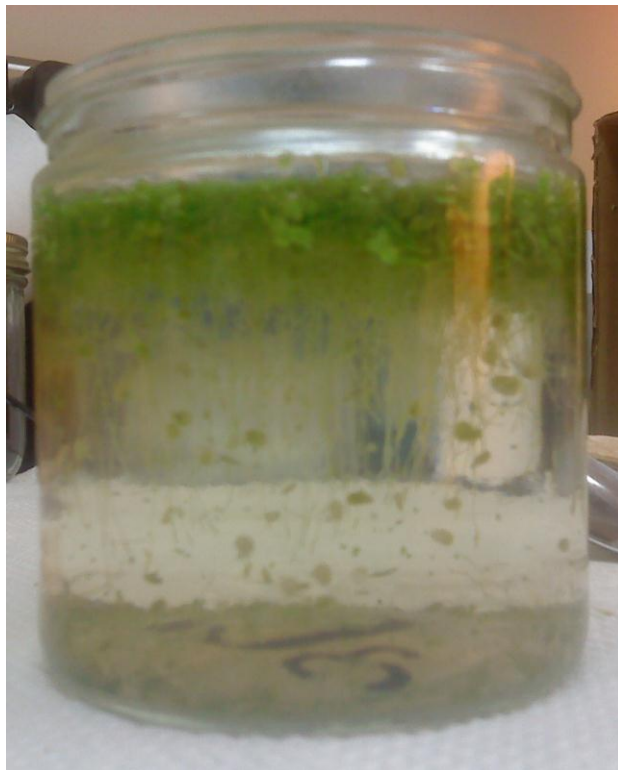
Figure 28. Light reactor with plants showing roots and senescing plants below the water surface—possible contributors to dissolved oxygen consumption.
