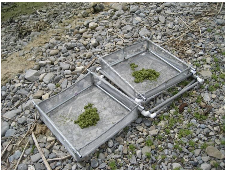
Figure 23. Duckweed inside of metal screened growth cells.
