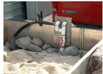
9. Keep the end of the clear hose in the tank because it is the return hose for Pump 1. Place the black hose near the location of the other valve using the large clip.
