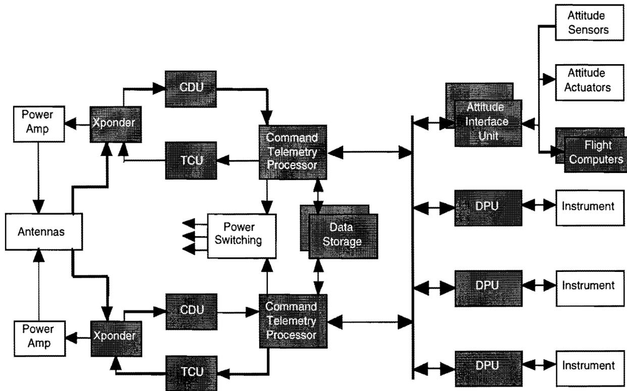
Figure 1. Simplified NEAR electronics block diagram.
