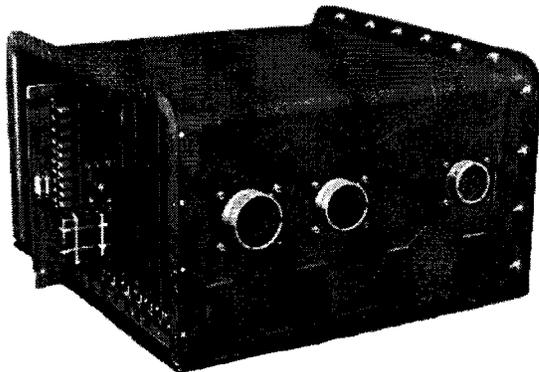
**Figure 3.** APL IEM Prototype Composite Chassis
