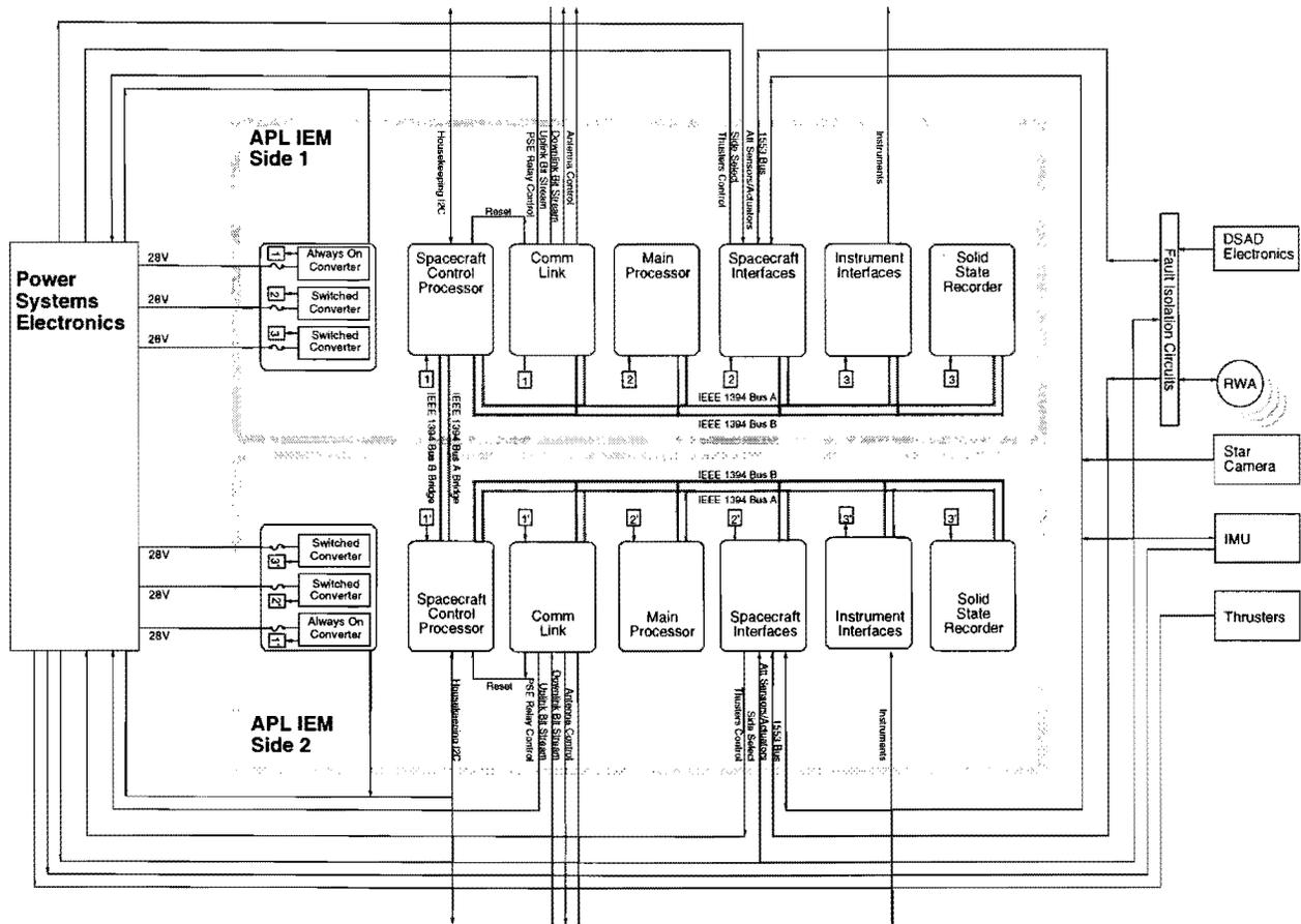
Figure 2. Deep Space APL IEM Configuration
