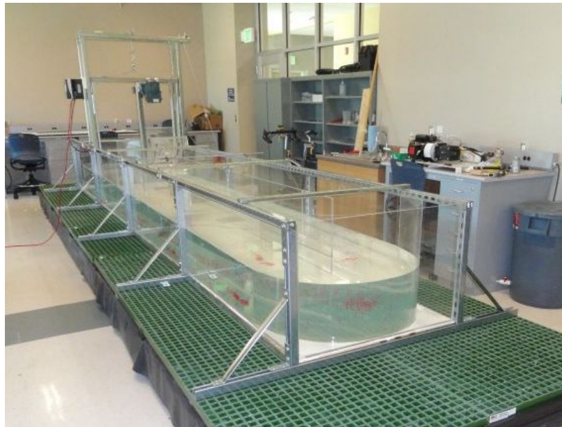
Fig. 3.1: Model Raceway constructed for fluid measurements
