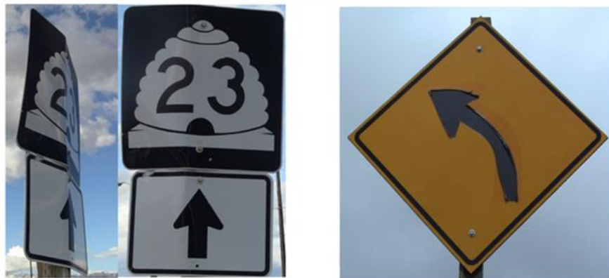
A. Bending Damage
