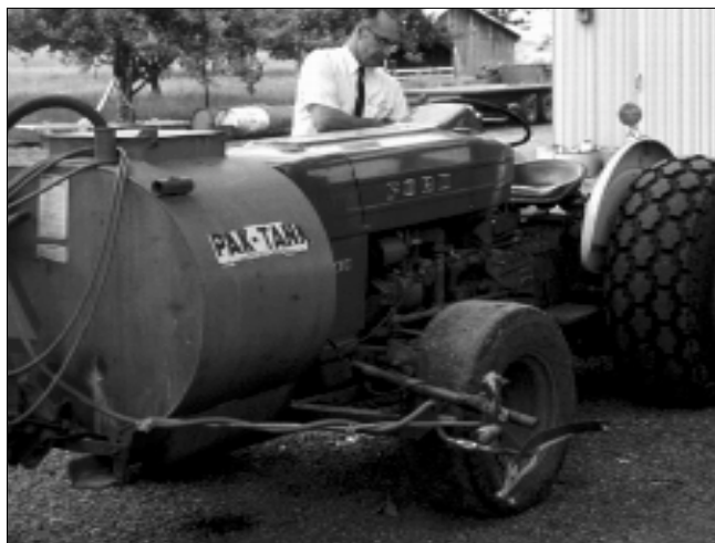
PAK Tank herbicide sprayer
