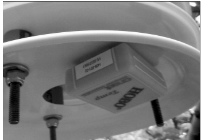
HOBO data logger in shelter
