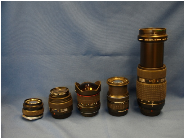
Figure 4. This photo shows different lenses. From left to right, 50mm prime lens ( f/1.4-16 ), 50mm 2:1 macro lens ( f/2.0-22 ), 8mm fisheye lens ( f/3.5-22 ), 14-42mm zoom lens (maximum aperture f/3.5-5.6 ), and 50-200mm zoom lens (maximum aperture f/2.8-3.5 ).
