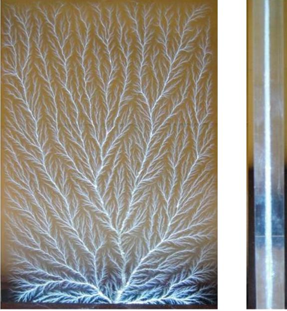
Fig. 1. Front (Left) and side (Right) views of a Lichtenberg discharge tree. The white line (Right) indicates the narrow distribution of deposited charge from a  $\sim 1$  MeV electron beam at  $R \approx 3$  mm in a PMMA sample.
