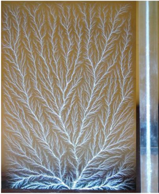
Figure 1. Front (Left) and side (Right) views of a Lichtenberg discharge tree. The white line (Right) indicates the narrow distribution of deposited charge from a ~1 MeV electron beam at R \approx 3 mm.
