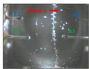
Figure 7. Photograph of nucleate boiling on a braided wire.
