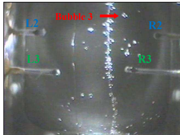
Figure 7. Photograph of nucleate boiling on a braided wire.
