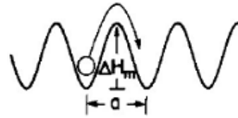
Fig. 1. Representation of carrier motion by way of hopping between potential wells. \Delta H_m and a correspond to well depth or trapped site binding energy and well separation, respectively [4,5].
