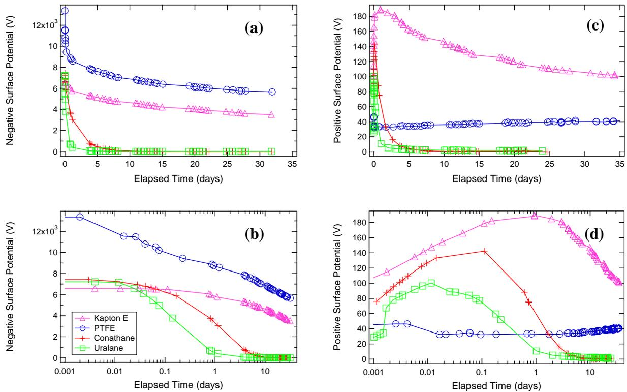
**Figure 4.** Surface potentials as a function of elapsed time for (a-b) 45 keV electron and (c-d) 1 MeV proton charged dielectrics. Note that (a) and (c) are linear plots while (b) and (d) have logarithmic time axes.
