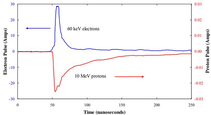
**Figure 2.** Comparison of dielectric current discharge pulse profiles from proton and electron exposure of Kapton E polyimide printed circuit board material.
