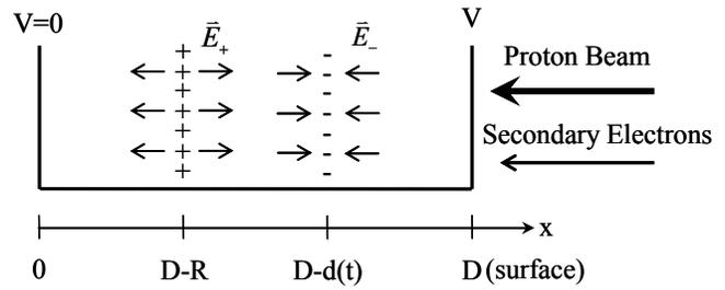
**Figure 5.** Simple charge slab model of charge within the sample. Shown are the grounded conducting plane at  $x=0$ , the fixed positive charge layer at  $x=D-R$ , the mobile negative charge layer at  $x=D-d(t)$ , and the dielectric surface at  $x=D$ . Also shown are the uniform electric fields from the charge layers. Diagram is not to scale.
