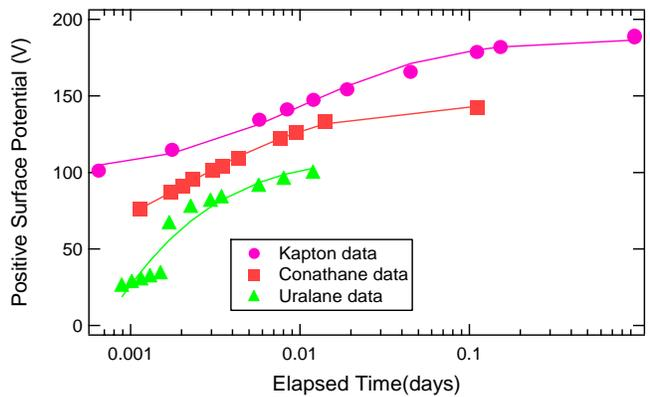
**Figure 6.** Surface potentials during the initial voltage rise as a function of elapsed time for 1 MeV proton charged dielectrics. The fit is based on Eq. (1), with  $d(t) \sim 1/t$ . Note the logarithmic time axes.
