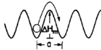
Fig. 1 Representation of carrier motion by way of hopping between potential wells. \Delta H and a correspond to structural elements of the material [4,5].
