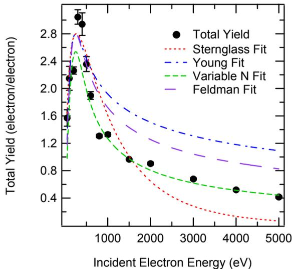
FIG. 10. In contrast to Fig. 8, reliable absolute total yields were obtained with flooding the sample between yield measurements. This yield curve for Al2219 ( $5 \mu\text{s}$  pulses with amplitudes 50 nA, each data point was the average of 10 pulses) is fitted with various analysis models. Best estimates for yield parameters are provided in Table 3.
