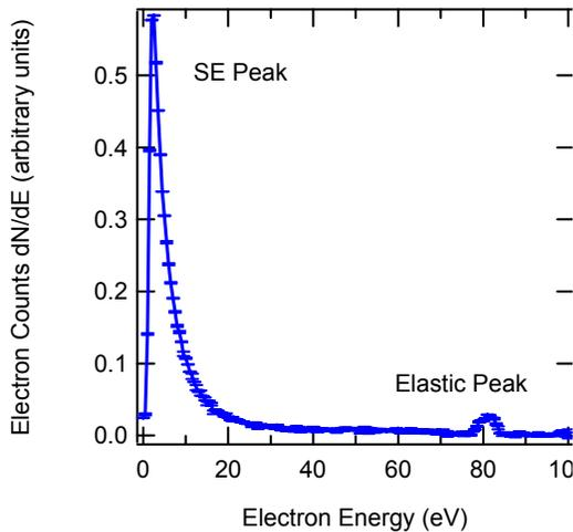
FIG. 1. Electron energy spectrum for Au, induced from a 80 eV electron beam. SE peak at  $2.3 \pm 0.5$  eV.
