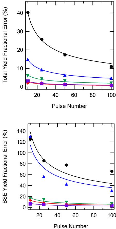
**Figure 9.** Fractional error as a function of pulse current magnitude and number of pulses for total yields (top) and BSE yields (bottom) using the low energy STAIB gun at 400 eV on conducting Ti at 10 nA (●), 25 nA (▲), 50 nA (▼), 75 nA (◆), and 100 nA (■) impulse magnitudes. Fits vary as the inverse of the root of the number of pulses.
