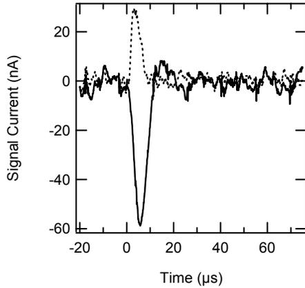
**Figure 4.** Measured sample (dot) and collector (solid) electron 5  $\mu$ s, 50 nA pulses on Au at 800 eV. Similar pulsed signals were obtained for stage and grid surfaces. Delayed rise and fall times were caused by system capacitance and ammeter response times.
