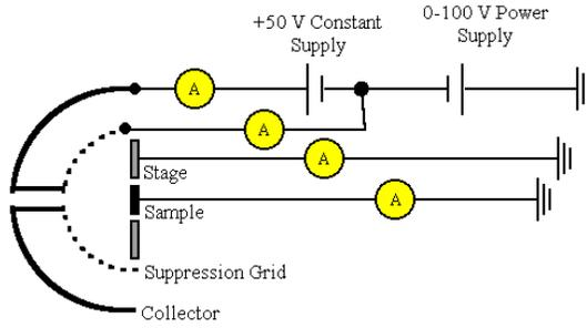
**Figure 1.** Basic schematic for DC- and pulsed-yield measurements. The incident electron beam enters through the detector aperture tube. Collector, retarding grid, sample, and stage currents are measured to calculate electron yields.
