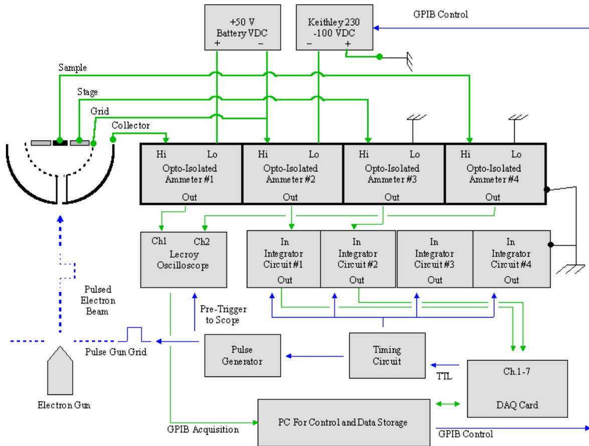
**Figure 3.** Pulsed-yield measurement block diagram for insulators.
