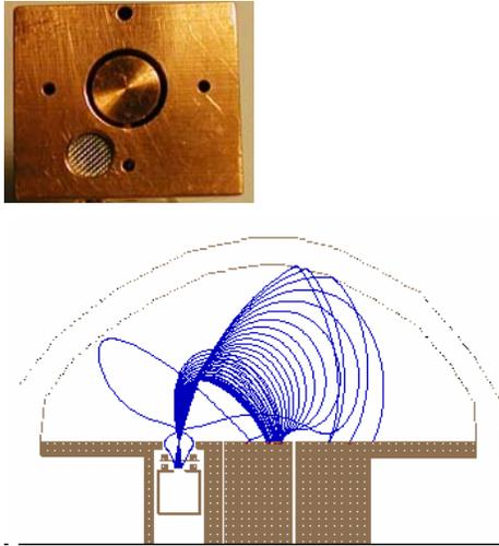
**Figure 7.** An electron flood gun sits adjacent to insulator samples and neutralizes positive surface charge. Top: a picture of the flood gun and sample. Bottom: a SIMION simulation of the flood gun inside the detector cavity next to a positively charged sample at +0.5 V and retarding grid at -1 V
