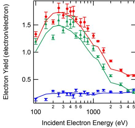
**Figure 10.** Comparison of pulsed total (●), SE (▲), and BSE (▼) yields with DC (solid lines) yields for Ti. Each data point is the mean of 10 pulses (standard error as bars), of time duration 5  $\mu$ s and magnitude 50 nA.
