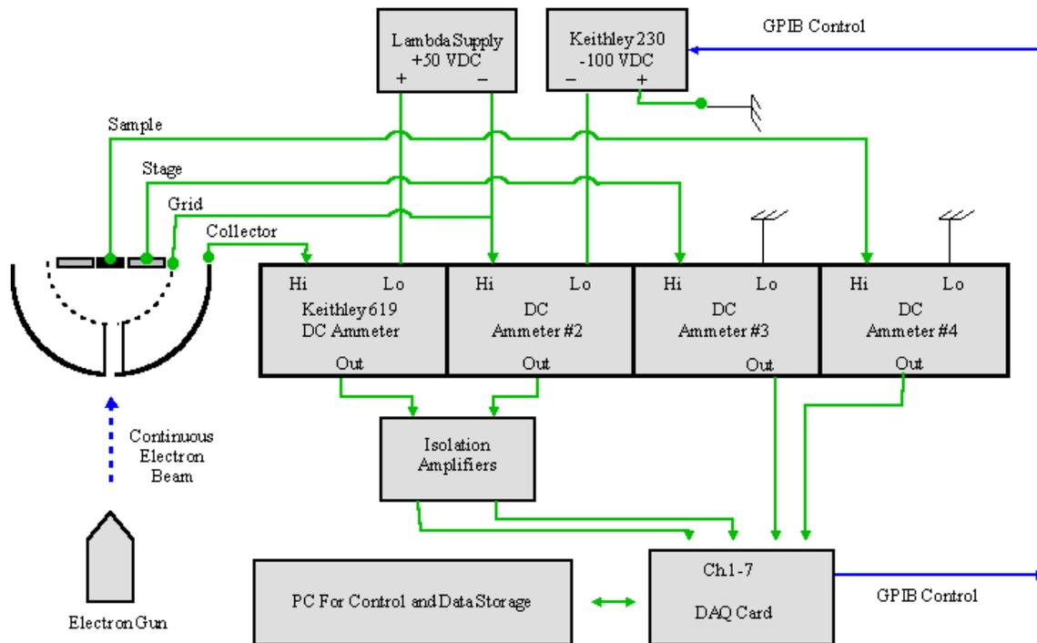
**Figure 2.** DC-yield measurement block diagram for conductors.
