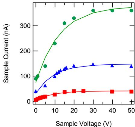
**Figure 8.** Flood gun current to a biased Au sample.  $I_{fil}=1.3$  A for all data; only the gun extraction potential is varied from 4 V (●), 3 V (▲), and 2 V (■). Sample current ranges from 5.5 nA to 75 nA at a 0 V sample potential, and from 42 nA to 380 nA at saturation.
