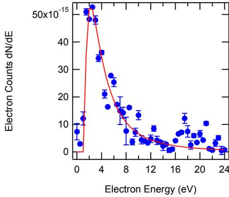
**Figure 11.** Pulsed-yield SE spectra on Ti at 400 eV. Data is fit with the Chung and Everhart model. Each data point is the mean of 10 pulses (standard error as bars), of time duration 5  $\mu$ s and magnitude 50 nA.
