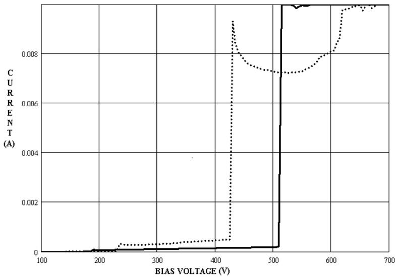
**Fig.8.** Two I-V curves are shown for the experiments for which glow discharges have been observed. The initiation voltage varies from 420 V to 510V. Cutoff at the 10 mA current is caused by the power supply limitation (Top of graph).
