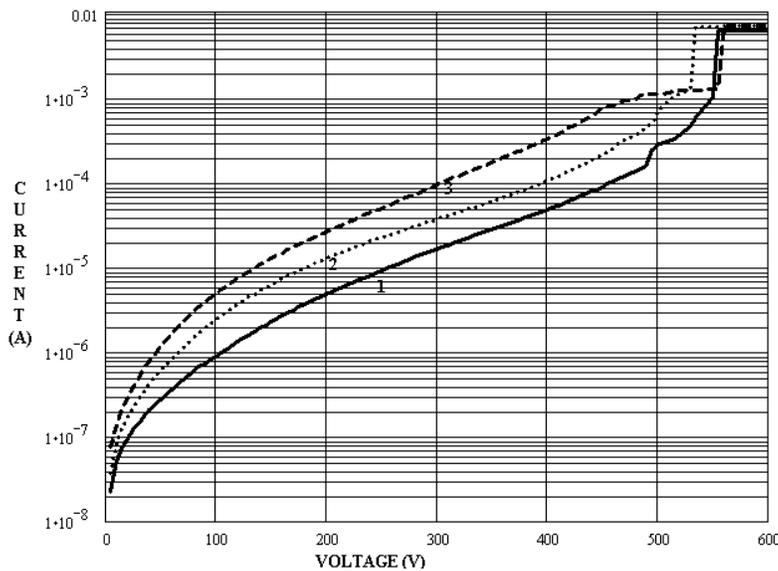
**Fig.13. Three I-V curves, measured for the anodized aluminum plate. The snapover initiation is clearly visible at voltages just above 100 V. The inception of a glow discharge at 530-550 V results in the sharp current increase. Numbers 1, 2, and 3 indicate the measurement sequence.**
