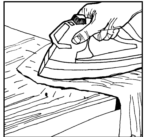
Figure 1. Using Steam and Heat to Remove Dents
